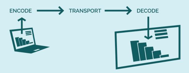
The three building blocks of every screensharing wireless presentation system: encode, transport and decode.
