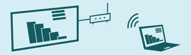
A common deployment of hybrid systems is to route all signals over the WLAN, so that users continue to have access to network resources in addition to the presentation system.
