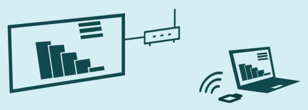
Hardware systems use a sender that plugs into the client device with either an HDMI or USB interface.
