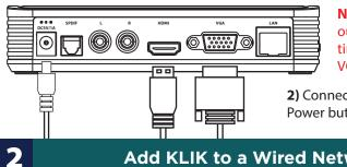
**NOTE:** Only one video output will be active at a time. Use either HDMI or VGA but not both.
